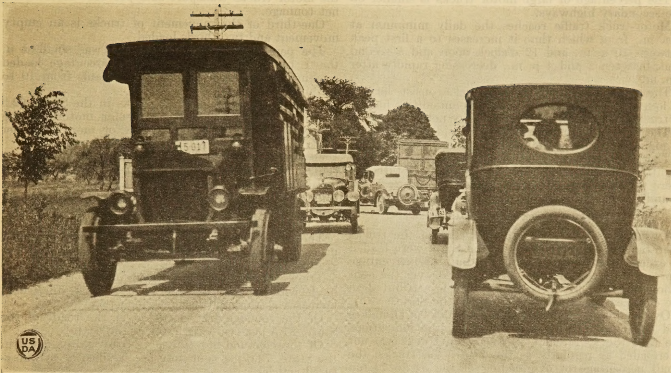
Traffic on the Boston Post Road near New Haven, Conn. Illustrating the retardation of passenger vehicles by motor truck traffic.
